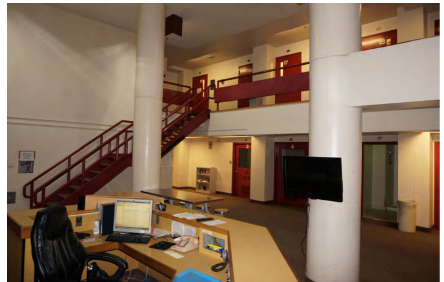
Figure 40: The officers' station in a typical housing unit has numerous blind spots and lacks visual access to much of the mezzanine level.
